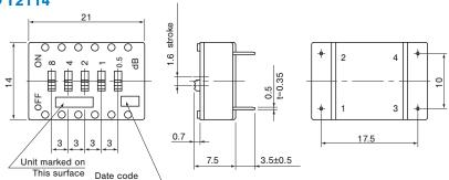
Unless otherwise specified, tolerance: ± 0.3 (Unit: mm)
