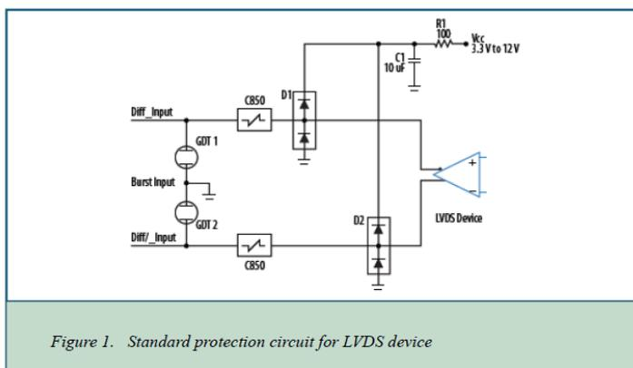
Figure 1. Standard protection circuit for LVDS device
