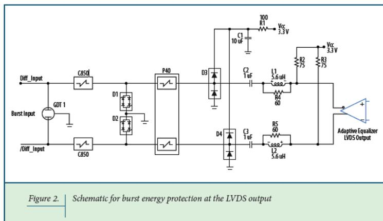
Figure 2. Schematic for burst energy protection at the LVDS output
