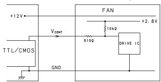
$V_{\text{CONT}}$  is above 2.6 V  $\cdots$  Fan should run full speed.
