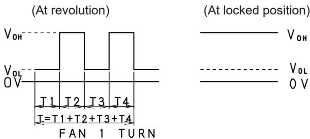
Remark: At locked position, output becomes  $V_{OH}$  OR  $V_{OL}$ .
