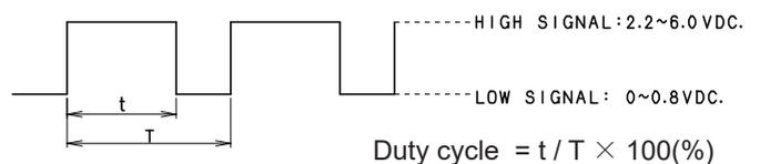
The frequency for control signal of the fan shall be able to accept at 15 kHz-30 kHz.
