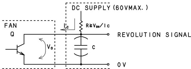
Remark: As for measuring  $V_{OL}$ , it is necessary to put a low pass filter which is constructed of R and C. The time constant of  $R \times C$  is to be more than 24 $\mu$ s.
