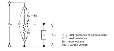
In the above diagram, if the load impedance is infinitely large, the output voltage ratio of the potentiometer will be proportional to the resistance change ratio.
