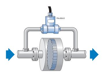
• Pressure sensing for water vapor
