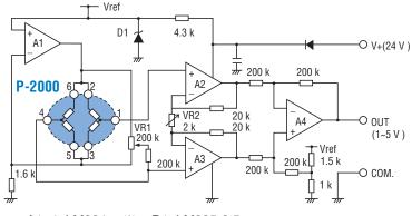
lepha In case of being required the improvement of accuracy, high accuracy amp. such as LT1014 is recommended
