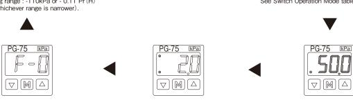
Press (M) button once. Both SW1 and SW2 LEDs will turn off and the Digital filter setting will be displayed. Set the value in the same manner. Response time: (F-0, 1, 2, 3, 4): (5, 25, 250, 1000, 2000)ms F-0 (5ms) is set prior to delivery.
