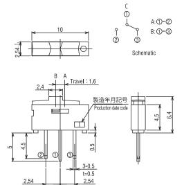
Unless otherwise specified, tolerance: ± 0.3 (Unit: mm)
